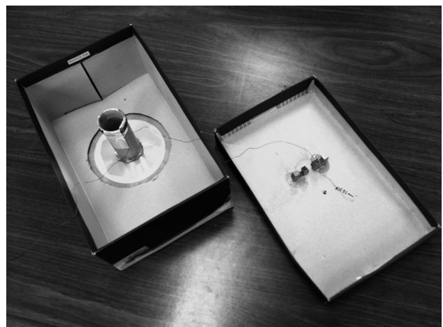
FIG. 3. Construction of the simplified shoebox speaker, showing how the assembly may be opened up to inspect the internal components.
