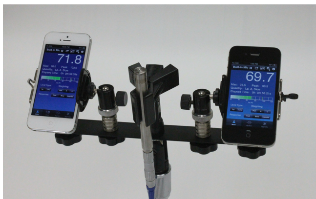
Fig. 1. (Color online) The SoundMeter app on the iPhone 5 (left) and iPhone 4S (right) compared to \frac{1}{2} -in. Larson-Davis 2559 random incidence type 1 microphone (center).
